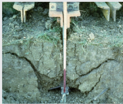
Figure 3. The soil disturbance produced by a tine working below its critical depth (left) and that produced by a winged subsoiler (right)
