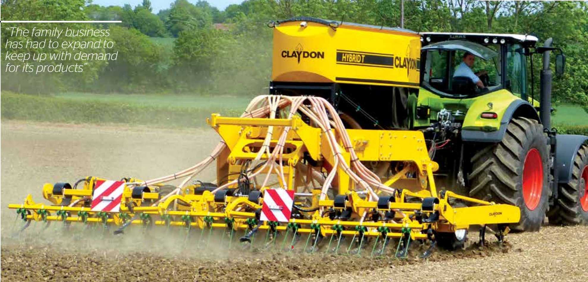
Two-metre wings fold down in field to give a 6m working width
