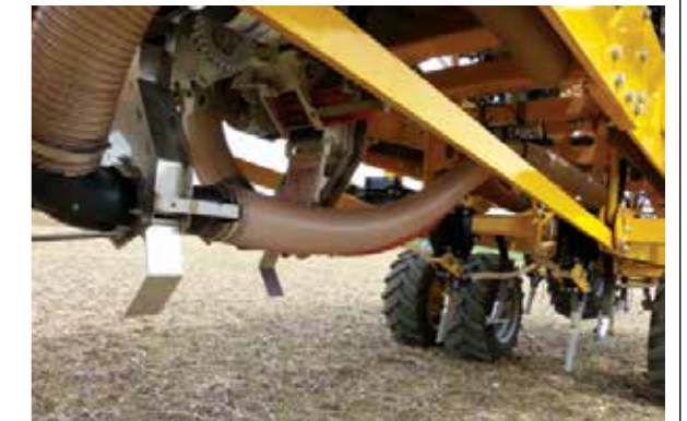
Below: Seeding tines are fed by pipes from the 5500-litre hopper
