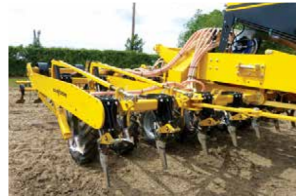
Far left: Front breaker tines allow minimal soil disturbance
