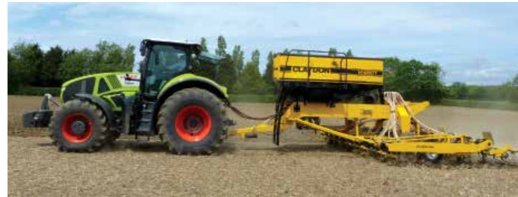
Bottom: Four wheels support the drill while in transport
