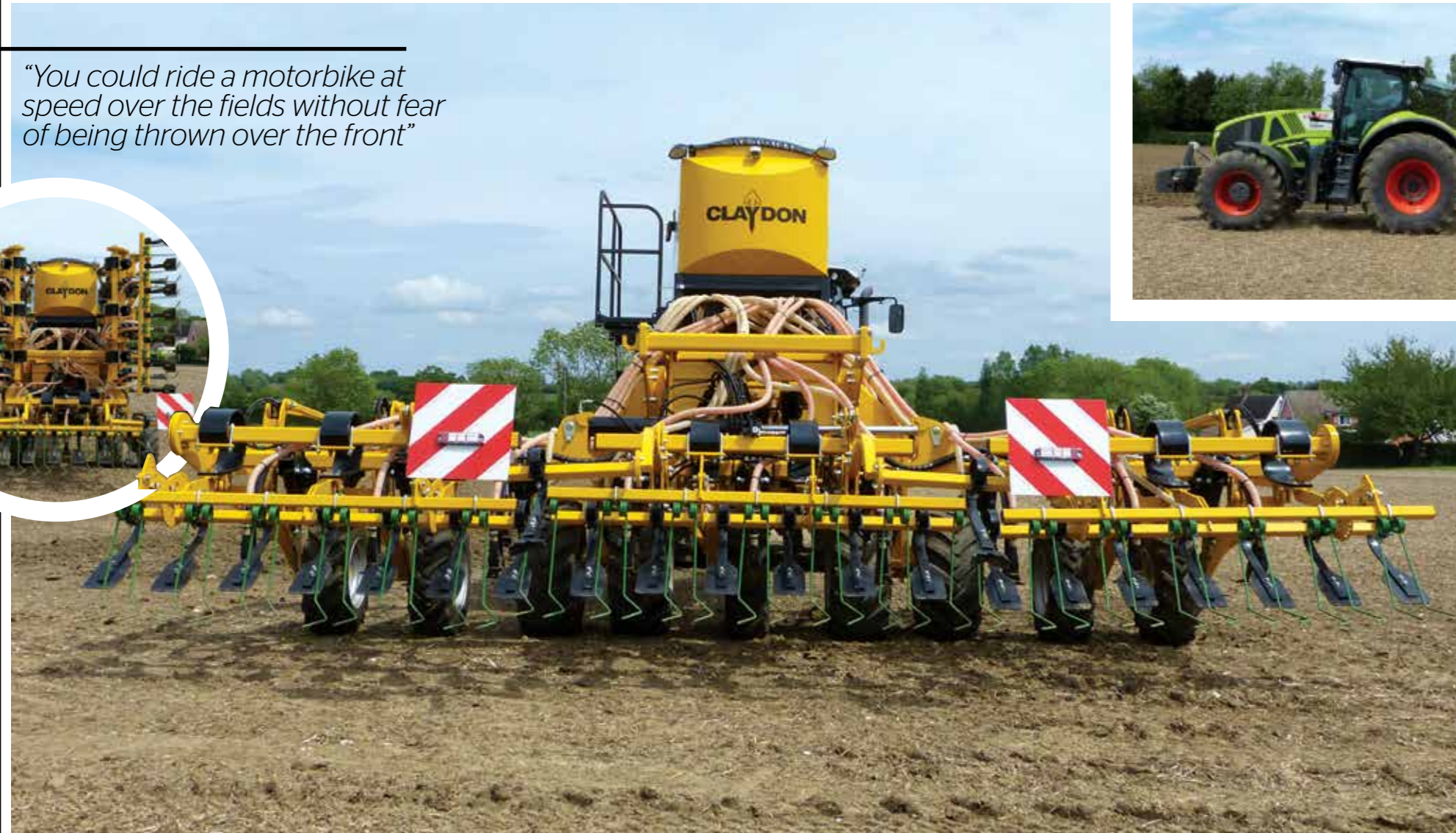
Inset: Folded, the Hybrid T meets 3m transport widths
